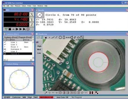
In order to quickly and directly compare the actual status and nominal status, import the parts drawing in DXF or IGES format, and place it over the video image.
