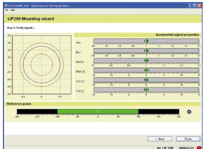
Commissioning using PWM 20 and ATS software
